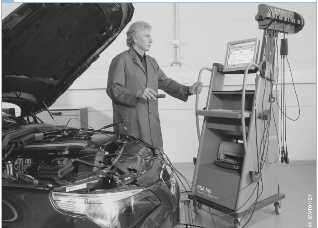
1 Diagnosis on a vehicle with a diagnosis tester
